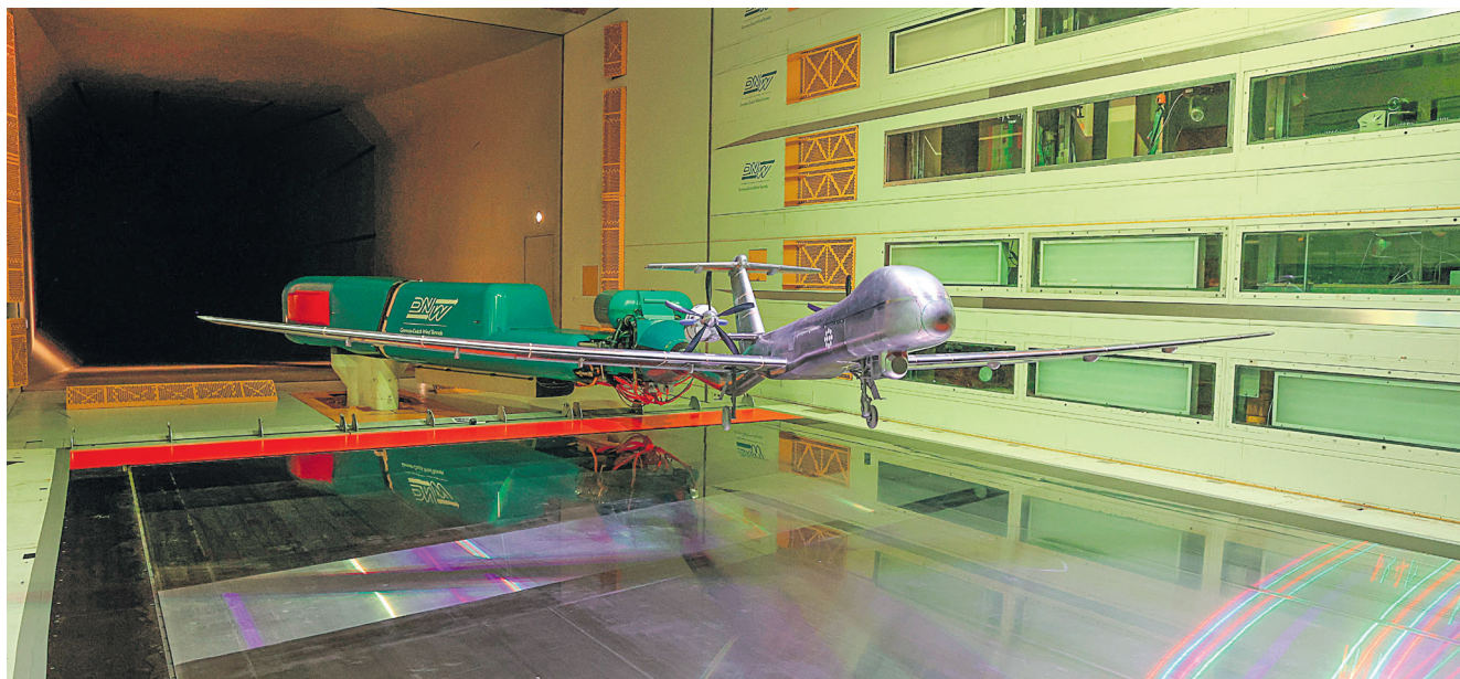
Scale 1/5 Eurodrone mock-up in the wind tunnel test
